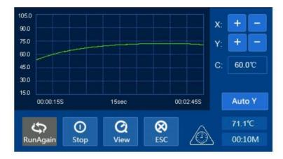
Press "Run", the unit will start to heat up to the desired temperature, and the message below will appear on the display. When the temperature has reached the desired level, press "Start" to continue.
