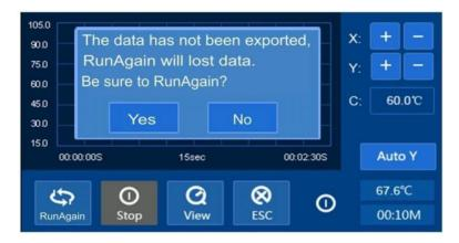
Press "Yes" to restart the program, the data stored in the device will be permanently erased (replaced by thenew data). Press "No" to exit the start-up, the device will ask you to insert a USB key to export the data.
