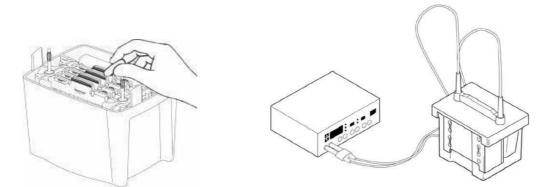
9. Disassemble the sandwich when the electrophoresis ends, take out the membrane and continue the next step. Use the neutral detergent to rinse the electrophoresis tank, blot clip, macroporous sponge, and then again use the ion-removing water to rinse.
