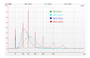
Figure 1. Size Distribution of mRNA Fragments (Agilent 2100 Bioanalyzer)
