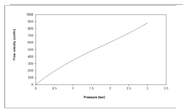
**Pressure-flow property of the IEX media:** The base matrix was packed to a 32 mm i.d. column with the final bed height of 15 cm. The mobile phase was deionised water. The test was conducted at room temperature.
