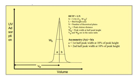
If the column is packed according to the instructions described above typical values obtained for Protein A Sep Fast resin should be:
