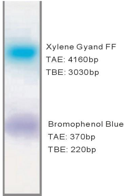
Electrophoresis of tracking dyes in 6x Gel Loading Dye
